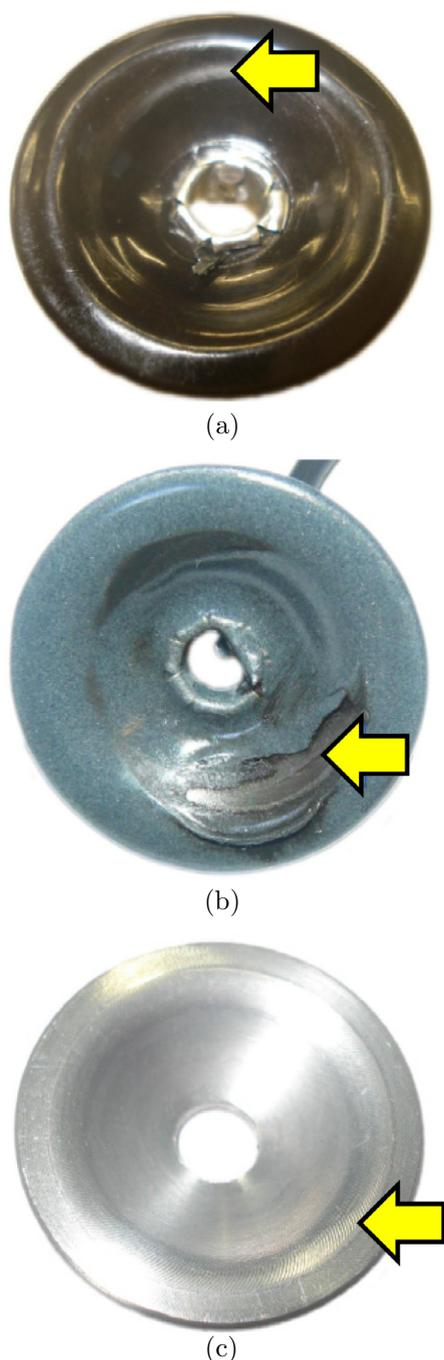
**Fig. 12.** Failed upper bearing coated with Rilsan (a), Loctite Nordbak 7227 (b), and anodized aluminum (c).
