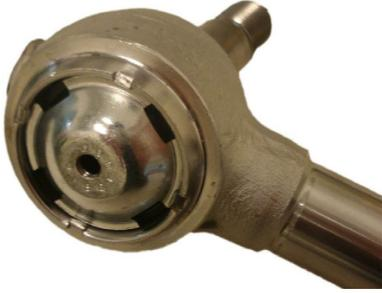
**Fig. 6.** Prototype of the ball joint including the wear sensor.
