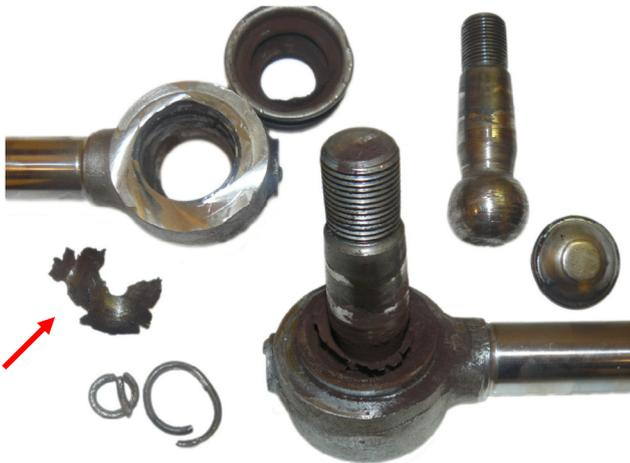
**Fig. 1.** Ball joint at the end of an endurance test performed without lubricating grease. The arrow highlights the completely failed conical upper bearing.
