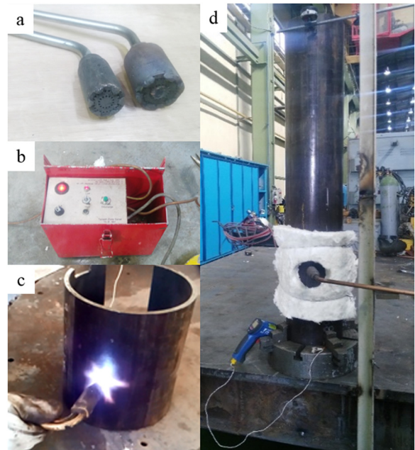
Fig. 16. Pipe wide heating test. (a) Torch heads, (b) spot welder, (c) half pipe calibration test, (d) main test.
