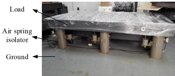
Fig. 8. Experiment platform supported by six air spring isolators.
