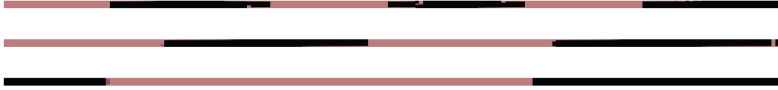
Fig. 9. Optimal solutions of the visco-elastic layer of the 2D sandwich beam (black: x_e > 0.99 ) for the compliance criteria, from bottom to top: \tilde{x}_{500 \text{ Hz}}^c , \tilde{x}_{1000 \text{ Hz}}^c , \tilde{x}_{2000 \text{ Hz}}^c .
