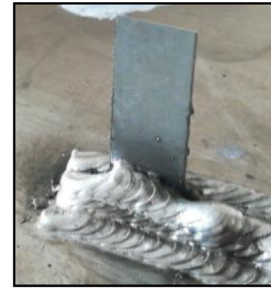
Fig. 18. Steel strip completely inserted between several layers.
