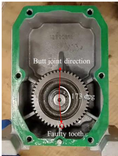
Fig. 16. The angular difference between the faulty gear tooth and the 'butt joint'.
