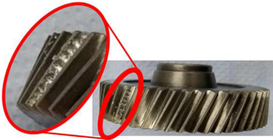
Fig. 12. The faulty gear used in the test of Case 2
