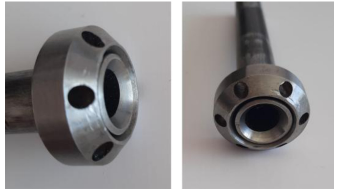
Fig. 12. The flared workpieces hydraulic tube end and fitting.
